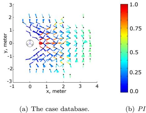
Fig. 3. The figure shows the values stored in the CBR system after completion of 20 test runs. Each dot represents a position of the test person in the robot coordinate frame. The facing direction of the test person is shown by the extending line, while the level of interest ( $PI$ ) is indicated by the color range of the line.
