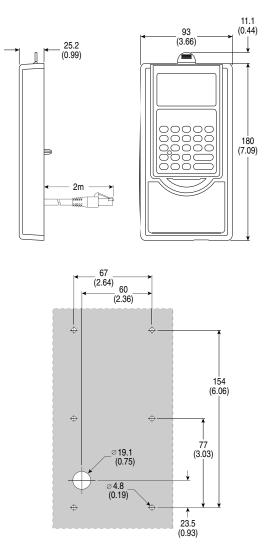
Figure B.14 NEMA Type 1 Bezel – Dimensions are in millimeters and (inches) Catalog Number: 22-HIM-B1
