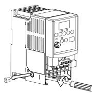
**Important:** Tighten screw after jumper removal.
