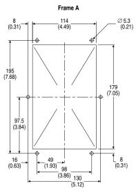
Figure B.4 PowerFlex 4 Cutout Dimensions – Dimensions are in millimeters and (inches)
