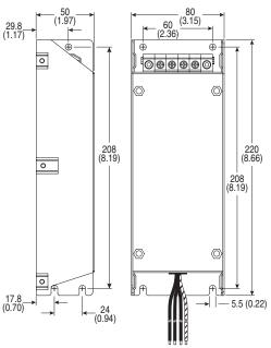
Figure B.9 Frame A EMC Line Filters – Dimensions are in millimeters and (inches) Catalog Numbers: 22-RF5P7-AS, -AL; 22-RF9P5-AS, -AL; 22-RF010-AL
