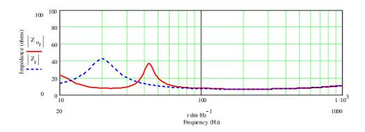
Woofer displacement is very well controlled. The blue dotted line is the driver in IB:
