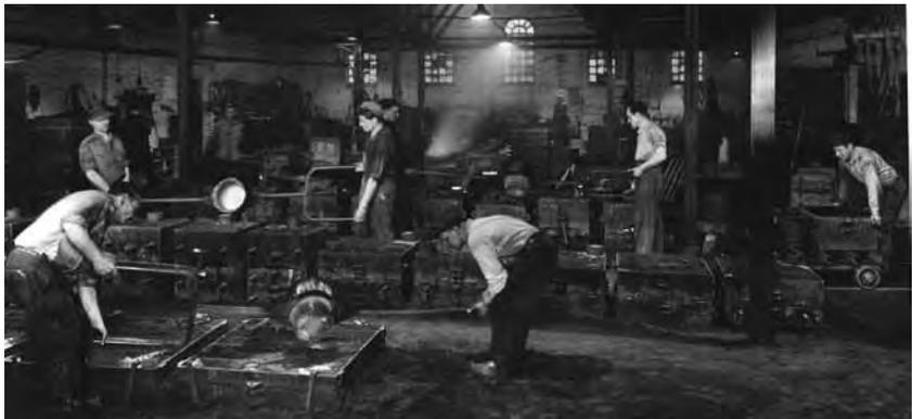
*The bell in the photograph has just been taken out of the mould and is about to be adjusted so it looks and sounds good. The mould, which is built into the wall, can be seen in the background. Photograph by Clausen, 1958.*
