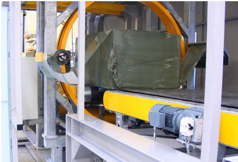
STEP 2: Vertical wrapping in the vertical ring stretchwrapper.
