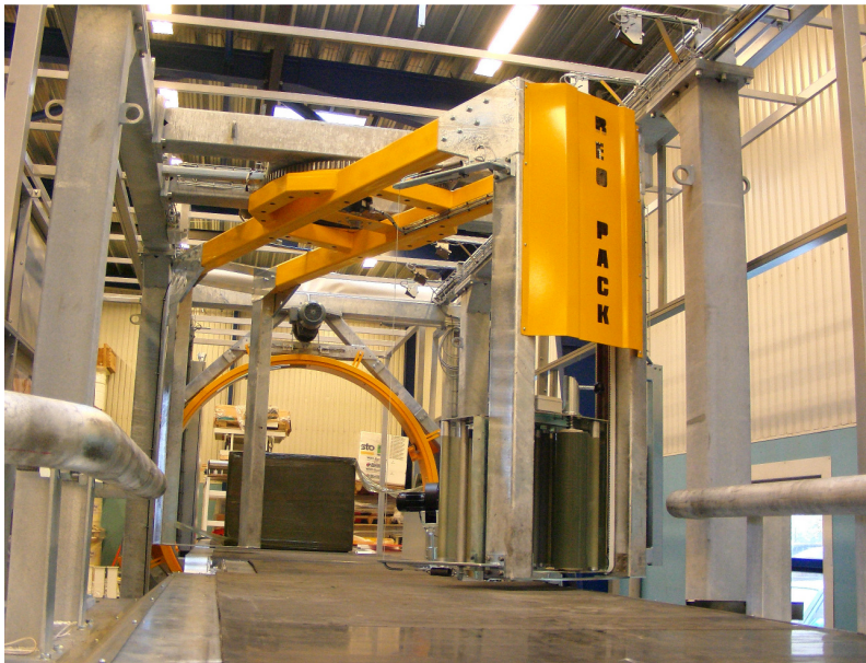
STEP 1: Horizontal wrapping in the swingarm stretchwrapper.
