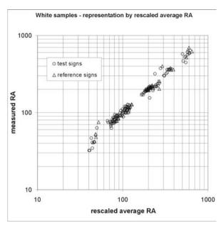
Figure 6: Actual R<sub>A</sub> values versus model R<sub>A</sub> values for white samples.
