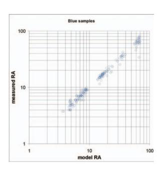
Figure 8: Actual R<sub>A</sub> values versus model R<sub>A</sub> values for blue samples.
